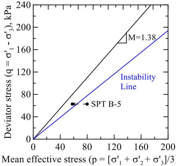
**Fig. 13. Comparison of instability line, critical state locus, and reduction in effective stress of segment 5 due to seismically induced pore-water using the piezometric data in P3.**
