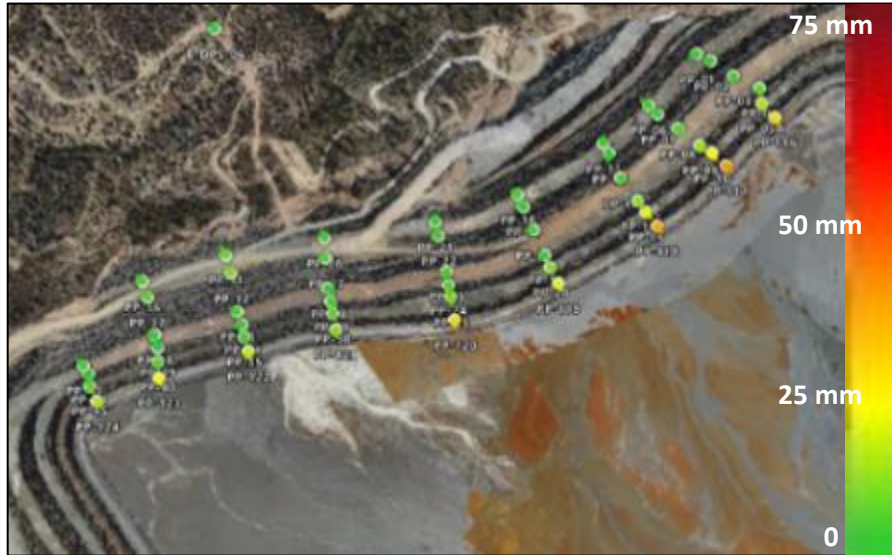
Prisms Location on the TSF (Vaguada Norte)
